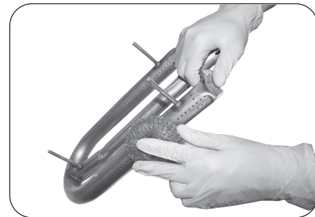
Fig. 4-2 Tubular burner cleaning
