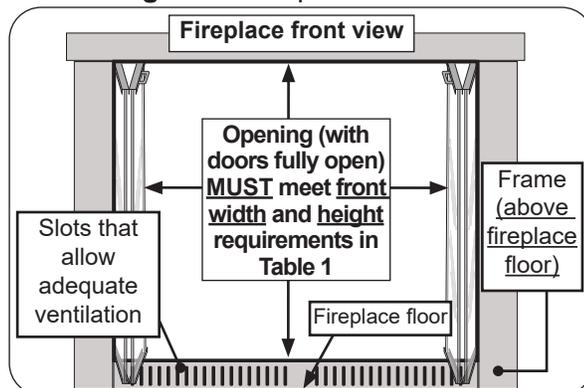
**Fig. 5-2** Glass doors frame ventilation (if applicable)
