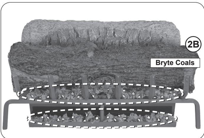
Separate half of the supplied bryte coals into small pieces, and evenly place them over the glowing embers in the middle ember bed as shown. Repeat this process for the remaining (second half) of bryte coals over the bottom ember bed.
