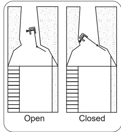
**Fig. 6-2** Damper open / closed
