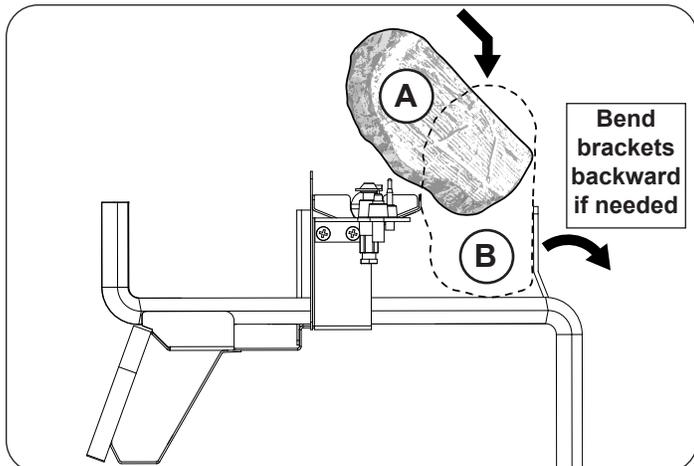
**Rear log placement detail:** First place the log, at an angle, against the rear burner brackets (see A). Then slide the log down into position – flat on the burner (see B).
