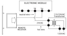
The remote control receiver can be connected, in series, to a 24VAC transformer to the TR (transformer) terminal on the electronic module. Connect the hot wire from the 24VAC transformer to either of the wire terminals on the remote receiver. Connect another wire (included) between the other receiver wire terminal and the TH (thermostat) terminal on the electronic module.
