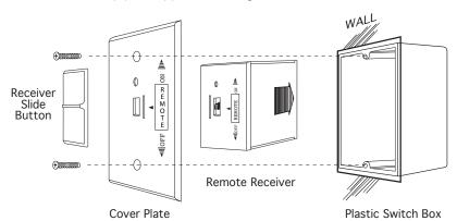
Position the receiver as shown in diagram to the left with lower tab on cover plate inserted into groove of receiver (Make the LEARN hole on cover plate properly aligns with remote receiver) Pull receiver up and snap into top tab of cover plate.
