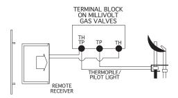
Operation of the remote receiver is similar to that of a thermostat in that both turn the gas valve on and off based on input signals. A thermostat's input signals are different temperatures. The remote receiver's input signals come from the transmitter.
