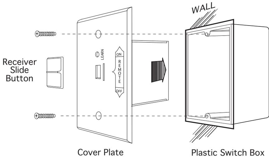
**NOTE:** The remote receiver will only respond to the transmitter when the 3-position slide button on the remote receiver is in the REMOTE position. If the system does not respond to the battery transmitter on initial use, see LEARNING TRANSMITTER TO RECEIVER, and recheck battery positions in the remote receiver.
