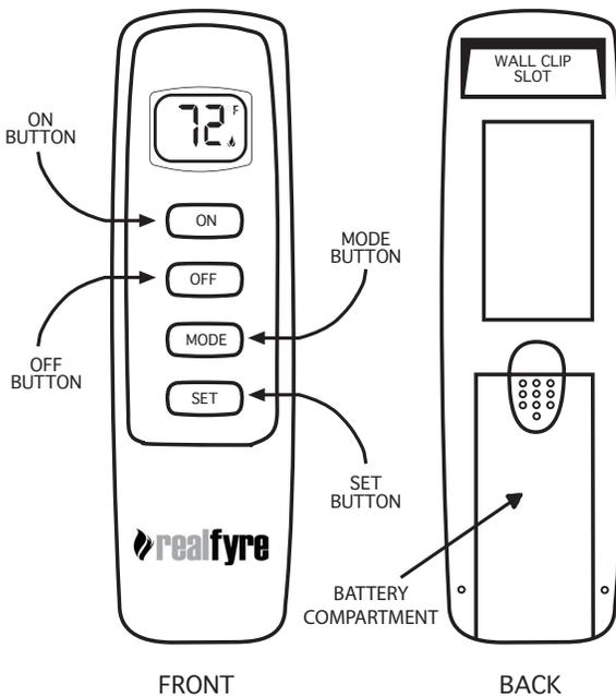
This remote control SYSTEM offers the user a battery-operated remote control that operates most millivolt gas valves used in some heater rated gas logs, gas fireplaces and other gas heating appliances.
