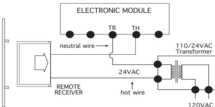
The remote control receiver can be connected, in series, to a 24VAC transformer to the TR (transformer) terminal on the ELECTRONIC MODULE. Connect the hot wire from the 24VAC transformer to either of the wire terminals on the remote receiver. Connect another wire (not included) between the other receiver wire terminal and the TH (thermostat) terminal on the ELECTRONIC MODULE.
