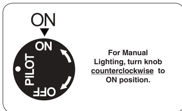
Fig. 13-1 Control knob detail (ON) - pan models
