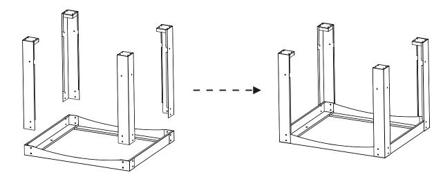
STEP 3 - Attach 2 x side shelf (7) to STEP 2 as shown on below diagram. Fix them using 16 x M8\*20 bolts (A),16 x Φ8 washers (B) and 16 x M8 nuts(D).
