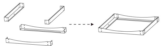
STEP 2 -Attach 4 x legs (8) to STEP 1 as shown on below diagram.
