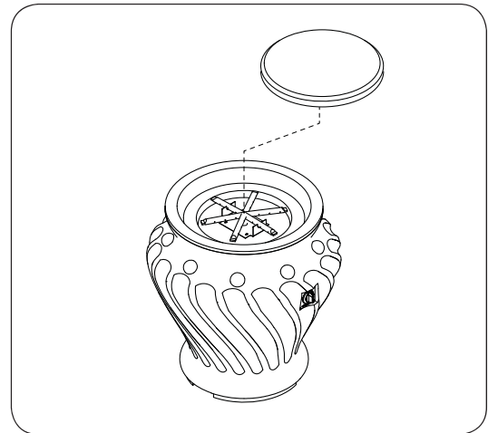
Fig. 18-1 GFRC cover placement
