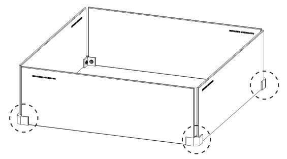
DO NOT overtighten screws. Tighten until snug. Overtightening can break glass.
