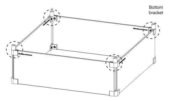
DO NOT overtighten screws. Tighten until snug. Overtightening can break glass.
