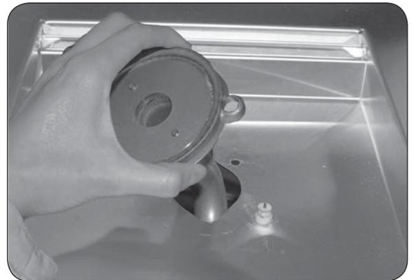
**Fig. 29-2** Remove burner
