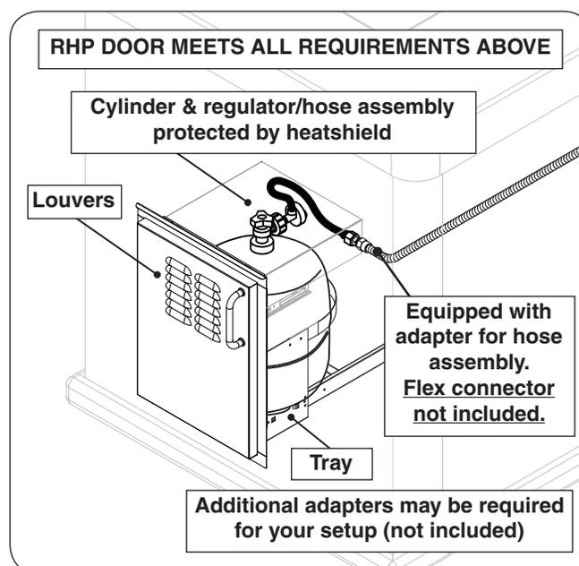
**Fig. 9-3** Optional AOG door w/ tank tray & louvers
