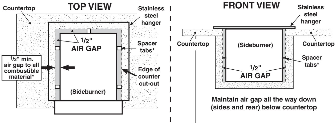
\* Use the spacer tabs located on the side and rear walls of the unit to assist in this required clearance.
