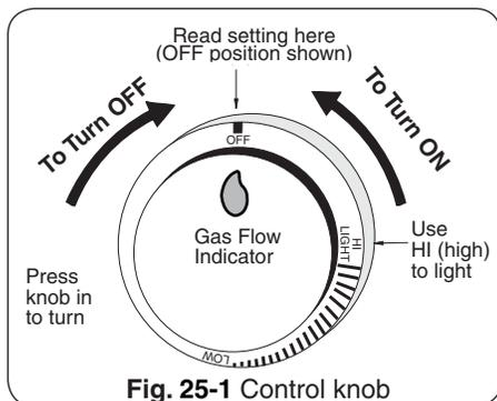
**Note:** If equipped, **DO NOT** turn on more than one valve at a time for either electronic or manual lighting.
