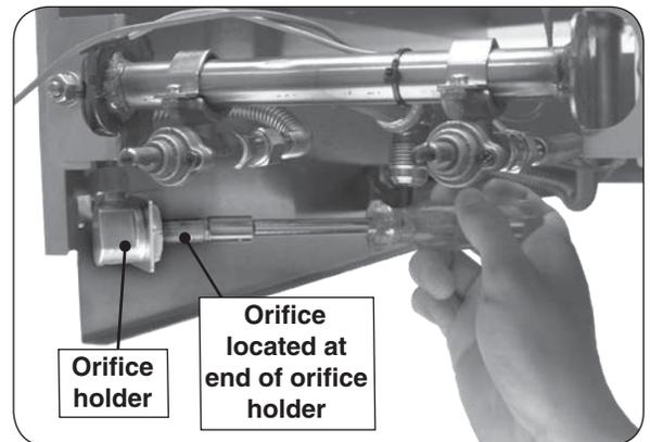
**Fig. 29-3** Orifice location
