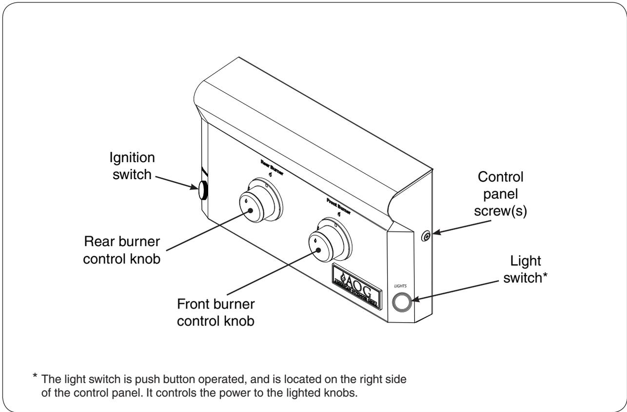
\* The light switch is push button operated, and is located on the right side of the control panel. It controls the power to the lighted knobs.
