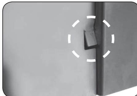
**Fig. 22-2** Tab slightly bent in for clearance
