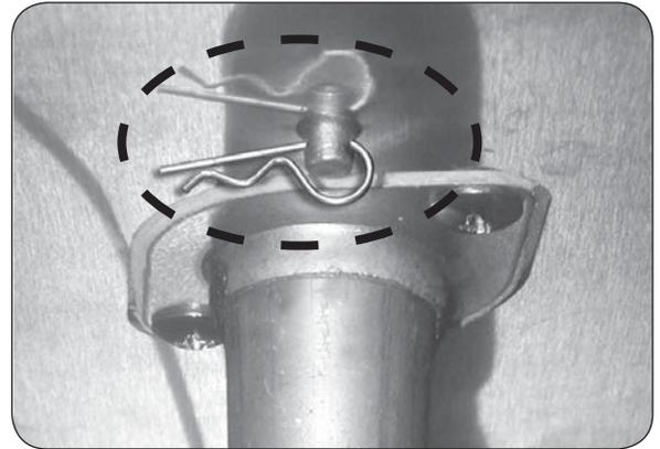
**Fig. 29-1** Remove burner clip
