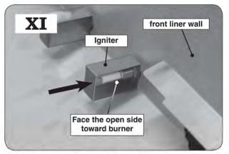
Install the new igniters (included in kit) into the front liner wall. Each igniter is to be placed from the interior of the grill, with the open side facing towards the burner. Fasten from the opposite side (behind face) using the included nut.
