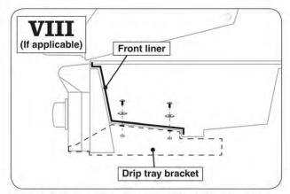
If the knock-outs were removed in step  ${\bf VI}$ , install the new drip tray bracket to the front liner using the supplied bracket screws, washers, and nuts. Fully tighten using a Phillips screwdriver and a  $^3/8$ " nut wrench.
