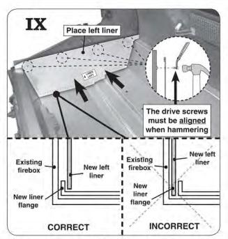
Place the left liner (item 4) as shown above. Rest the liner OVER the front and rear liner flanges (hiding the flanges) and ensure the 4 holes are aligned with the 4 grill wall rivets. To secure the liner, align each drive screw (included in kit) with the corresponding hole and carefully hammer each drive screw into the panel. Use needle-nose pliers to assist in holding the drive screws properly.
