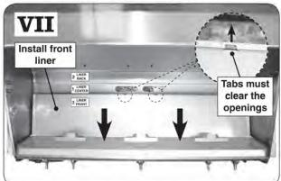
Place the <u>front liner</u> (item 3) ensuring it rests flat against the grill <u>front firebox wall</u>, and the two tabs (on center liner) extend up through the slots in the front liner.
