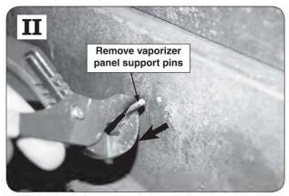
If vaporizer panel support pins exist on the <u>rear firebox</u> <u>wall</u> of the grill, remove those pins using pliers as the new burners (included in this kit) will provide support for the new vaporizer panels.
