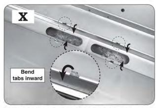
Using pliers, bend in the four tabs inward toward the middle of the center liner to lock the liner panels together.
