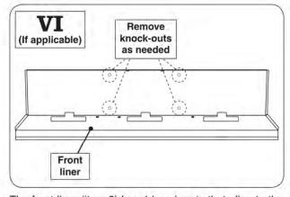
The front liner (item 3) has 4 knock-outs that align to the drip tray bracket below the unit once installed. If the old drip tray bracket was previously removed, remove the knock-outs using a flat head screwdriver. These new holes will be used to provide support to the new drip tray bracket.
