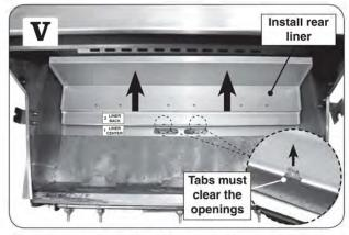
Place the <u>rear liner</u> (item 2) ensuring it rests flat against grill <u>rear firebox wall</u>. The two tabs (on center liner) must extend up through the slots in the rear liner.
