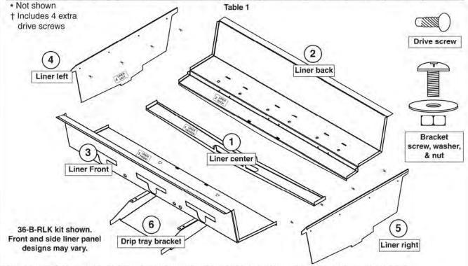
This firebox liner kit is for installation on AOG grills. Installation on a 36" unit is depicted in this instruction.
