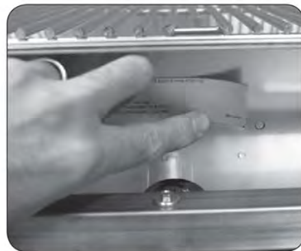
Fig. 4-3 Apply the conversion label
