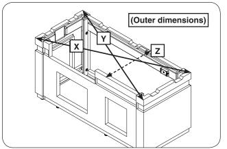
Fig. 8-2 Square unit (then tighten bolts)
