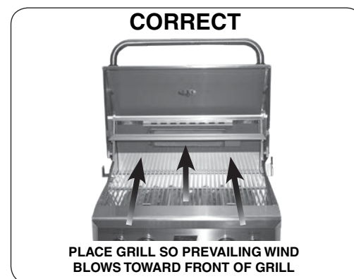
Fig. 10-3 Correct venting
