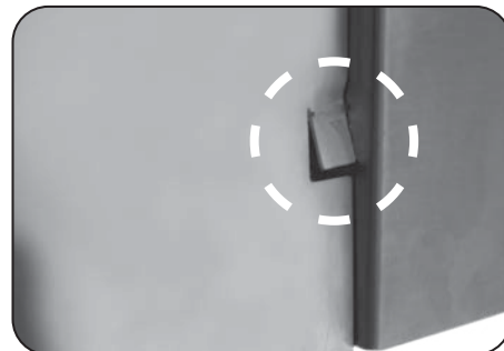
Fig. 19-2 Tab slightly bent in for clearance
