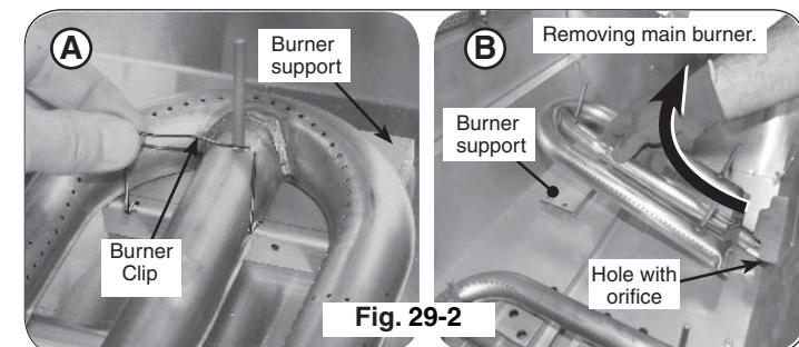
4. Use a  $\frac{1}{4}$ " hex deep socket nut driver to remove the exposed orifice. Access it through the hole in the forward firebox plate inside the grill (Fig. 29-2). Check orifice. If needed, replace it with the correct orifice for the new gas.
