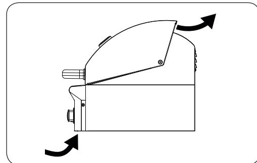
Fig. 10-1 Airflow diagram
