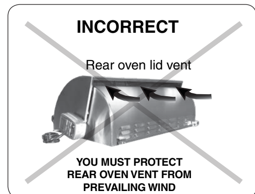
Fig. 12-3 Airflow direction - INCORRECT
