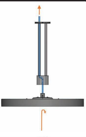
7. Fully insert additional 2 X Dome Head Screws (M4 - Length: 6mm) on both sides, and tighten all four screws, to lock heater in place.
